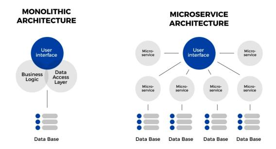
Microservices, in contrast, allow developers to break down the application into smaller, manageable services that can be developed, tested, and deployed independently. Each microservice can be built using different technologies and can scale independently based on demand. This decoupling of services leads to improved agility, as teams can work on different
